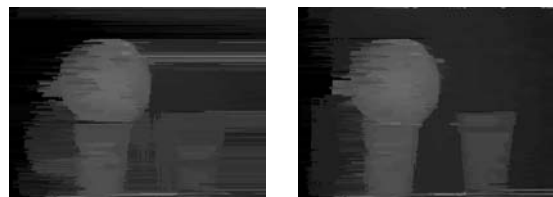
c) range image by dynamic programming d) range image by the proposed integration algorithm
